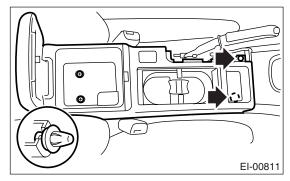
4) Disconnect the connector, and remove the console box.
