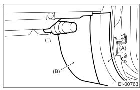
8) Remove the clip, and remove the glove box lower cover.
