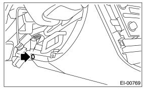
7) Remove the passenger side front inside scuff plate (A) and front pillar lower trim (B). <Ref. to El-60, REMOVAL, Lower Inner Trim.>
