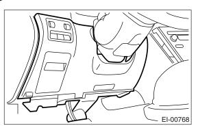
6) Remove the clip at the console side panel tip.
