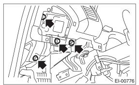
7) Remove the bolts at the side of passenger side instrument panel.
