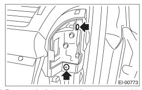
14) Remove the bolts securing passenger side airbag module to the steering support beam.
