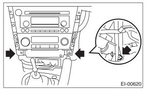
9) Disconnect each connector, and remove the instrument assembly.
