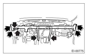
5) Remove the steering support beam bracket.
