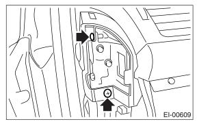
10) Remove the screw at the side of center console.
