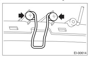
22) Remove the pawl, and remove the passenger's airbag module.
