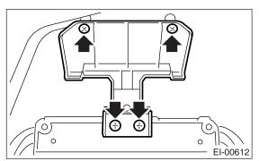
20) Loosen the screws to remove instrument panel matching pins.
