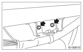
15) Disconnect the connectors, and remove the instrument panel from vehicle body.
