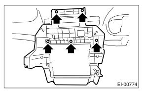
19) Loosen the screws to remove meter bracket.
