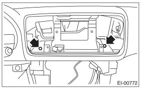
13) Remove the screws at side of passenger side instrument panel.
