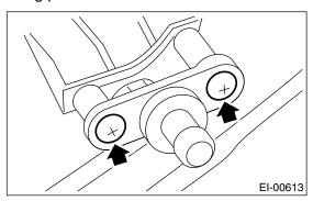
21) Loosen the screws to remove glove box striker.
