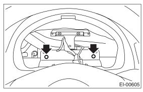
9) Remove the driver side instrument panel side cover, and remove the screws.
