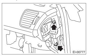
8) Loosen the bolts on the center console side.
