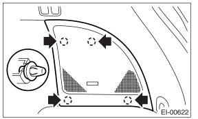
8) Remove the screws (A) and bolts (B), and remove the quarter lower trim.
