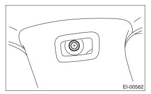
4) Remove the bolts (A), and remove the quarter trim (front).
