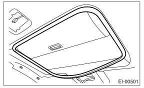
10) Remove the clips and each harness, pull out the rear center seat belt, and remove the roof trim.
