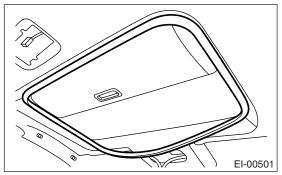
14) Remove the clips and each harness, and remove the roof trim.
