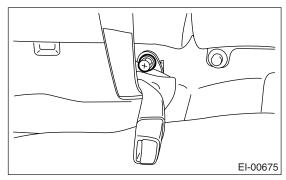
6) After disconnecting the high-mounted stop light harness connector (A) and removing the five clips, remove the rear shelf trim with pulling it frontward.
