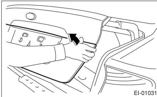
3) Remove the trunk lid garnish in the order from the end of it, by accessing it through the gap between trunk lid garnish and trunk lid panel.
