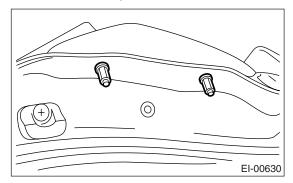
4) Remove the nuts, disconnect each connector, and remove the rear gate garnish.
