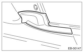
8) Remove the bolt, and remove the front fender panel.
