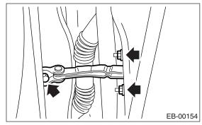
13) Remove the front door. <Ref. to EB-17, FRONT DOOR ASSEMBLY, REMOVAL, Front Door.>
