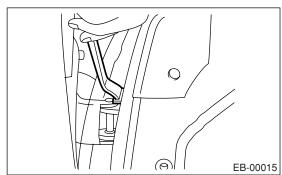
8) Remove the door hinge from vehicle.
