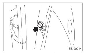
7) Remove the door-side bolts for upper and lower hinges to remove front door panel.
