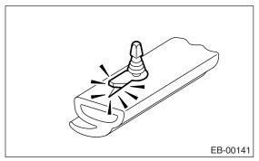
12) Remove the bolts and nuts to remove door checker.
