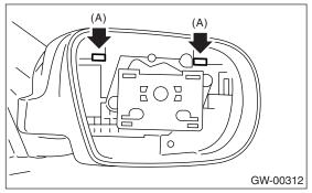
3) Pull the scalp cap frontward of door mirror, remove the upper side clips (A) and lower side hooks (B), and then remove the scalp cap.
