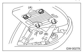
4) Disconnect the mirror heater connector from the end of mirror. (Model with mirror heater)
