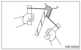
6) Pull the wire ends alternately to cut off the adhesive part.
