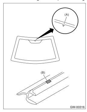
9) Apply two types of primers to the adhesive layer of glass using sponge.
