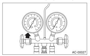
8) Leave it at least 5 minutes, and then check the low-pressure gauge reading for any changes.
