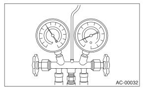
19) If the HFC-134a source is empty, close the high-pressure valve, close the valve on the can tap, and replace the HFC-134a source with a new one to restart the operation.
