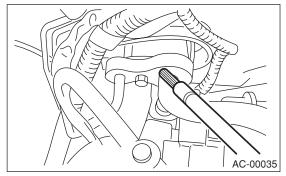
9) Visually check the rubber area of the flexible hose for cracks.
