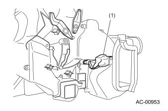
(1) Evaporator sensor connector
