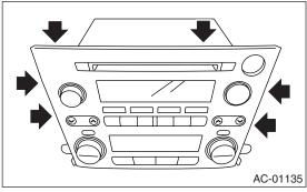
3) Using a fine flat tip screwdriver, remove the ten hooks gradually in the order of both sides, lower and upper side.
