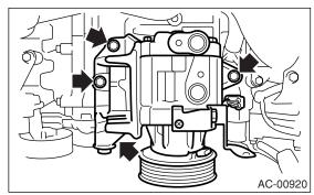
10) Remove the bolts, and then remove the bracket from compressor.
