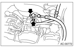
8) Disconnect the compressor harness from body harness.
