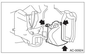
4) Remove the bolts securing expansion valve and pipe in engine compartment.
