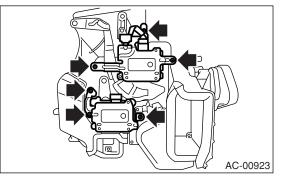
3) Disconnect the connector, remove the screw and remove the pipe cover and evaporator sensor.
