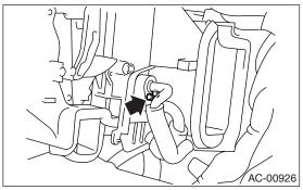
6) Remove the screws and clip to remove the evaporator cover.
