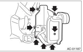
7) Pull out the evaporator (A) in the direction of arrow.
