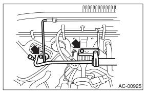
5) Remove the bolt which holds the pipe to evaporator.
