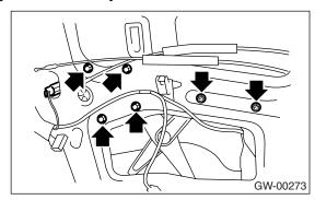
4) Remove the screws to remove motor assembly.
