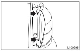
3) While pressing the portion (A), insert your finger or flat-tip screwdriver wrapped with tape into the clearance (B) to remove pawls in the order of (C), (D), (E), and remove the rear combination cover.
