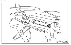
9) For glass stroke adjustment, install the ST to glass, close the door, and raise the glass with regulator until positional relationship between glass and weather strip becomes as shown. And secure the glass so that the upper stopper correctly touches the glass holder.
