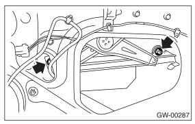
7) Remove the rear sash retaining nuts (A) and move rear sash (B) backward.
