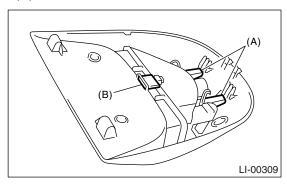
5) Disengage three claws and remove the lens (A).
