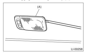
3) Disconnect the harness connector and remove the lens.
