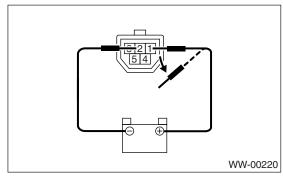
4) Connect the battery and confirm that the wiper motor stops at automatic stop position after the wiper motor operates at low speed again.
