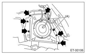
5) Disconnect the harness connector and detach woofer.
