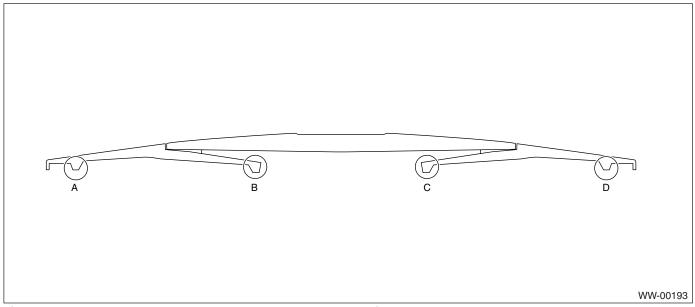
1) Insert the wiper rubber through the claw B.
