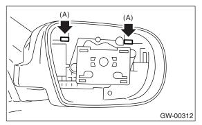
3) Pull the scalp cap frontward of door mirror, remove the upper side clips (A) and lower side hooks (B), and then remove the scalp cap.
