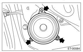
4) Disconnect the harness connector and remove rear speaker.
