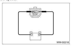
2) When the battery is connected to the terminal of connectors, confirm that the wiper motor operates at high speed.
