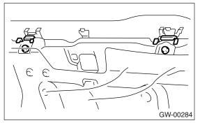
4) Remove the clips (A), and remove the front end and rear end of weather strip.
