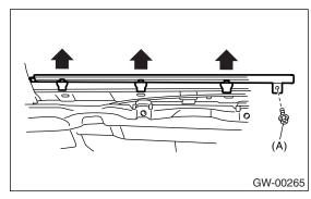
9) Remove the screws to remove guide assembly. 10) Operate the power window switch to move glass to position shown in the figure, and then remove the two nuts through service holes.
