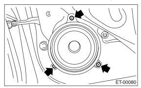
4) Disconnect the harness connector and remove front speaker.
