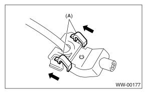
3) Remove the washer hose from washer nozzle.
