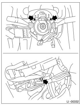
6) Remove the switch securing screw to remove combination switch.
