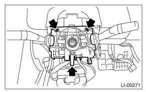
7) Disconnect the connector and remove the combination base switch assembly.
