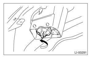
5) Remove the spring retainer then detach the fog light bulb.
