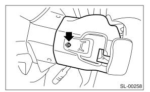
3) Remove the instrument panel lower cover. <Ref. to EI-56, REMOVAL, Instrument Panel Assembly.>
