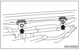
7) Remove the clips (A), and remove the rear end of weather strip.
