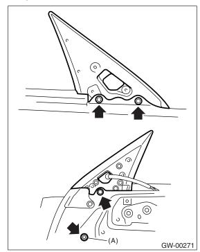
16) After adjustment, tighten the bolts and nuts.
