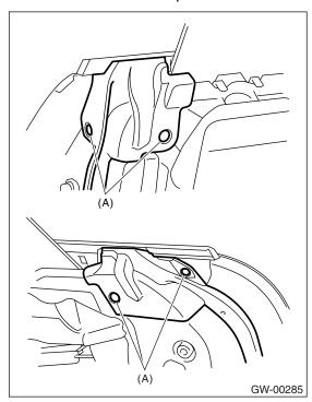
5) Loosen the two screws to remove weather strip outer.
