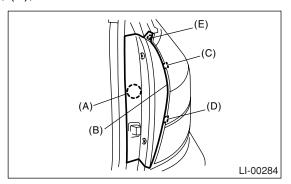
4) Remove the two bolts, and then detach the rear combination light by pulling it to the rear side of vehicle.
