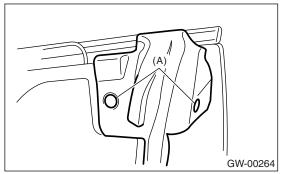
8) Remove the screw (A) from the rear end of weather strip outer to remove weather strip outer.
