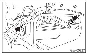
7) Remove the rear sash retaining nuts (A) and move rear sash (B) backward.
