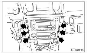
6) Disconnect the harness connector and antenna feeder cord, and then remove the audio.
