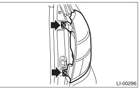
5) Remove the rear combination light after turning the socket of tail/stop light bulb and rear turn signal light bulb to remove the bulbs.
