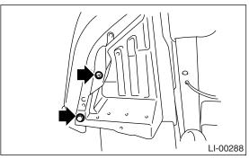
3) Disconnect the harness connector.4) Remove the mounting nuts and clips, and then detach the fog light assembly by pulling it.
