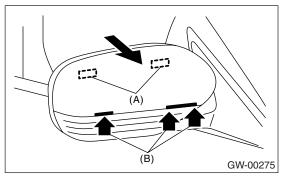
4) Insert the lower hooks (B) of scalp cap to door mirror and push the upper clips (A) in.
