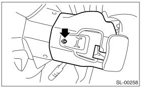
4) Remove the combination switch. <Ref. to LI-9, REMOVAL, Combination Switch (Light).> <Ref. to WW-6, REMOVAL, Combination Switch (Wiper).> 5) Remove the four screws and remove the roll connector.
