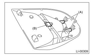
5) Disengage three claws and remove the lens (A).
