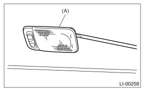
3) Disconnect the harness connector and remove the lens.
