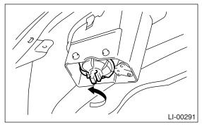
5) Remove the spring retainer then detach the fog light bulb.
