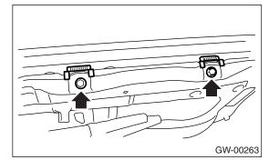
7) Remove the clips (A), and remove the rear end of weather strip.
