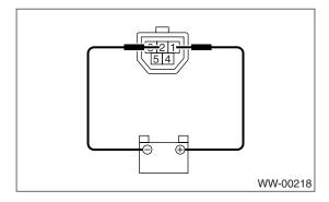
2) When the battery is connected to the terminal of connectors, confirm that the wiper motor operates at high speed.
