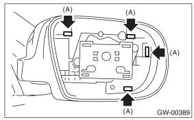
3) Pull the scalp cap frontward of door mirror, and then remove the scalp cap.
