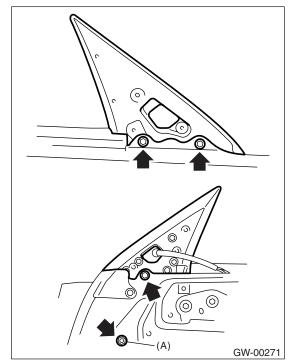
16) After adjustment, tighten the bolts and nuts.
