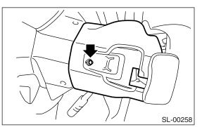
3) Remove the instrument panel lower cover. <Ref. to EI-56, REMOVAL, Instrument Panel Assembly.>
