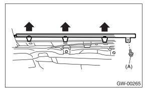
9) Remove the screws to remove guide assembly.10) Operate the power window switch to move glass to position shown in the figure, and then remove the two nuts through service holes.
