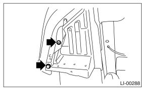
3) Remove the horn bracket mounting bolt (A).4) Disconnect the harness connector and remove the horn assembly (B).
