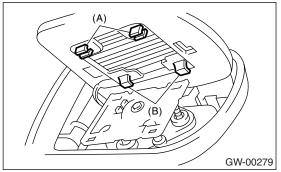
4) Disconnect the mirror heater connector from the end of mirror. (Model with mirror heater)
