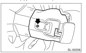
4) Disconnect the connector from combination switch.
