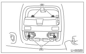
3) Disconnect the harness connectors and remove the spot map light.
