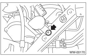
5) Remove the two bolts and one nut, hose, connector and washer motor cover, and then remove the washer tank.
