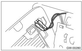
5) Catch the hooks (A) and install clips (B).
