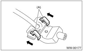
3) Remove the washer hose from washer nozzle.
