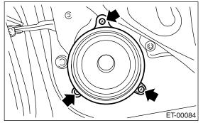
4) Disconnect the harness connector and remove rear speaker.
