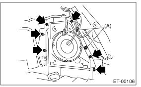
5) Disconnect the harness connector and detach woofer.
