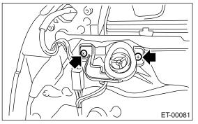
4) Disconnect the harness connector and remove tweeter.
