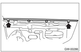
6) Operate the power window switch to move the glass to position shown in the figure, and then remove the two nuts through service holes.
