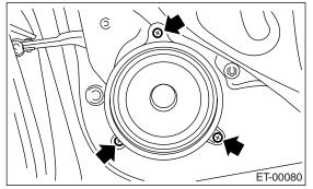
4) Disconnect the harness connector and remove front speaker.
