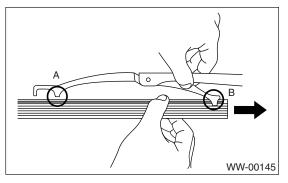
2) Insert the wiper rubber until its top end protrudes approx. 20 mm (0.79 in) from stopper D.
