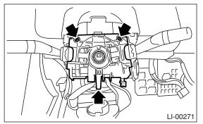
7) Disconnect the connector and remove the combination base switch assembly.
