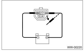
4) Connect the battery and confirm that the wiper motor stops at automatic stop position after the wiper motor operates at low speed again.
