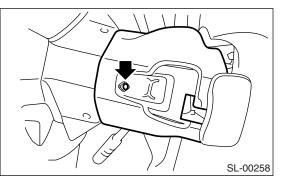
4) Disconnect the connector from combination switch.
