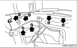
4) Remove the screws to remove motor assembly.
