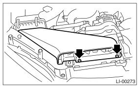
3) Remove the battery cover. (When removing the headlight bulb LH).
