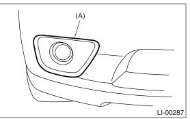
3) Disengage the two clips, and then turn over the lower mud guard.
