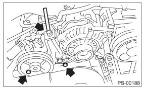
8) Place the oil pump bracket in a vise, and remove the two bolts from the front side of oil pump.
