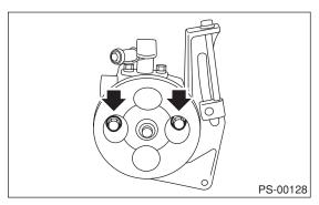
9) Remove the bolt from the rear side of oil pump.
