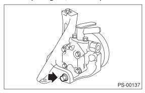
2) Tighten the bolts which hold the power steering pump bracket.
