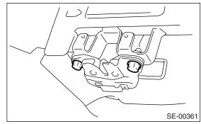
5) Loosen the screws to remove the armrest from backrest assembly RH.
