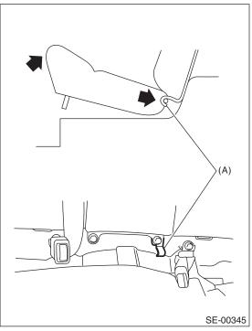
3) Remove the lower anchor bolt of rear center seat belt.
