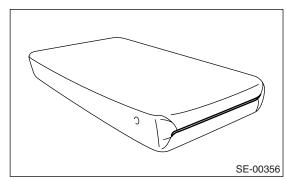
8) Remove the hook and hog ring, and then remove the headrest cover.
