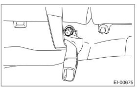
4) Remove the bolts which secure the bottom of backrest.
