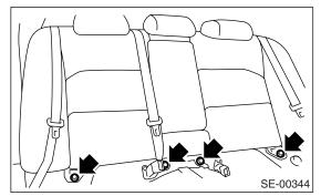
5) Remove the anchor part on backrest side from the hook on body side (A) while lifting up the backrest to detach it from vehicle.
