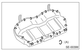
10) Remove the hog rings (A), and then remove the seat cushion cover.
