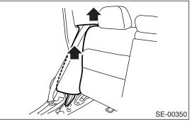
10) Remove the belt cover (A) from backrest shoulder cover, and then pull out the seat belt.
