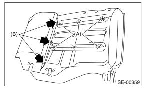
3) Remove the hog rings (A) on the front side of backrest, and then remove the backrest cover.
