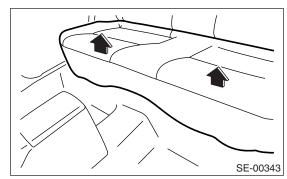
3) Remove the hook (A) by pushing it backward while lifting up the front side of seat cushion to detach seat cushion.
