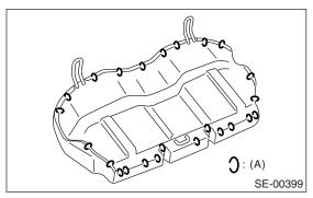
11) Remove the hog rings (A), and then remove the seat cushion cover.
