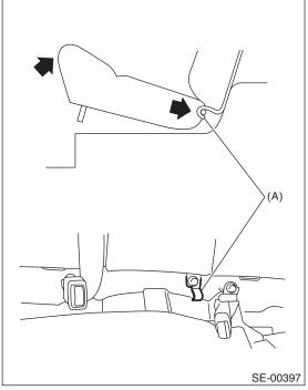
4) Remove the headrest, and then tilt the backrest forward.
