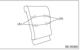
4) Remove the bolts, and then remove the backrest latch.
