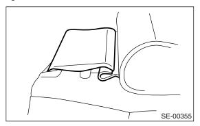
8) Remove the hook, and then remove the armrest cover.
