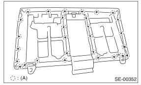
5) Remove the hog rings (A) on the front side of backrest.
