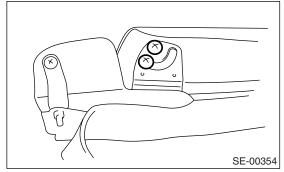
7) Remove the hook, and then detach the center through cover.
