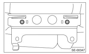
4) Remove the hog rings (A) on the rear side of backrest.
