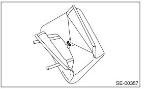
10) Remove the hog rings (A) on the rear side of seat cushion.
