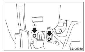
9) Remove the backrest shoulder with lifting it up.
