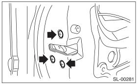
9) Remove the front door latch & door lock actuator assembly, and disconnect the connector.
