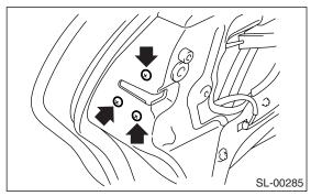
9) Disconnect the connectors, and then remove the rear door latch & door lock actuator assembly.
