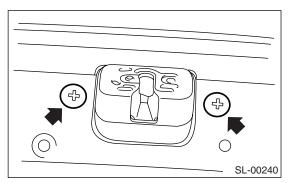
4) Disconnect the each connector and cable of rear gate handle.
