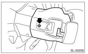
3) Remove the instrument panel lower cover. <Ref. to EI-50, REMOVAL, Instrument Panel Lower Cover.>
