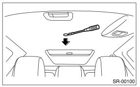
4) Insert the wrench securely until it touches the motor shaft edge.
