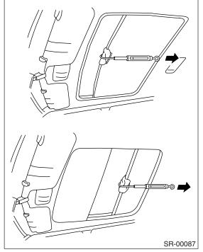
2) Pull the spring balance to measure moving load of the sunshade.
