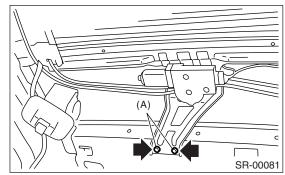
6) Remove the drain tube from frame assembly.7) Remove the frame bracket (A).
