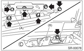
7) Remove the nuts, and then remove the frame assembly.
