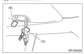
6) Remove the clips, and then drop the rear end of roof trim.
