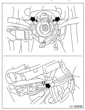
7) Remove the switch securing screw to remove combination switch.
