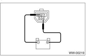
3) Connect the battery to terminals of connector, and remove the terminal connection with wiper motor rotated at low speed, and stop the wiper motor through operation.
