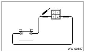
3) Connect the battery and confirm that the wiper motor stops at automatic stop position after the wiper motor operates at low speed again.
