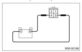
2) Connect the battery to terminals of connector, and remove the terminal connection with wiper motor rotated, and stop the wiper motor through operation.
